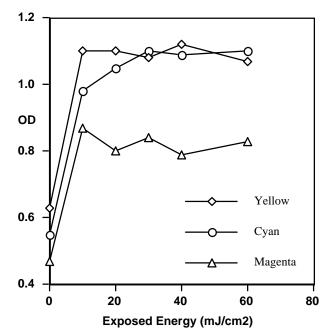
Figure 3. Water Immersion Test after Print/UV Exposure OD values of initial samples are Y:0.93, M:1.00, C:1.08, paper: PB paper (copier paper of Canon).
