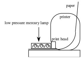
Figure 2. Printer with curing lamp
